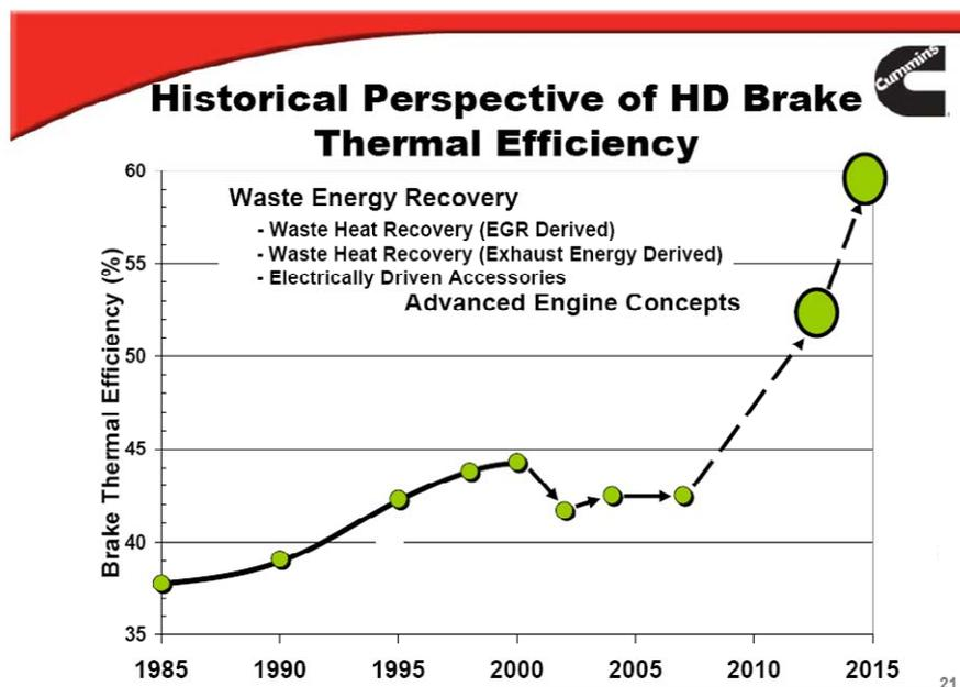
Figure 5.7. Projected increase in engine thermal efficiency (Eckerle 2007).
