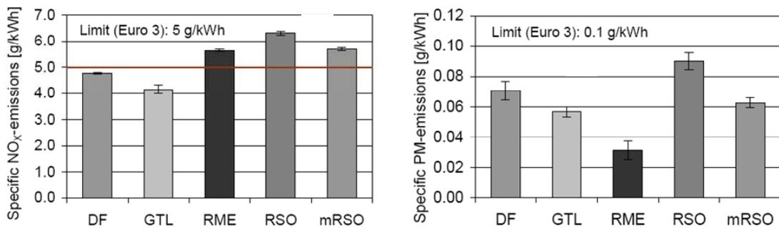
Figure 6.9. NO<sub>x</sub> and PM emissions with diesel fuel, GTL, RME and unmodified (RSO) and modified (mRSO) straight vegetable oil (Krahl et al. 2007).
